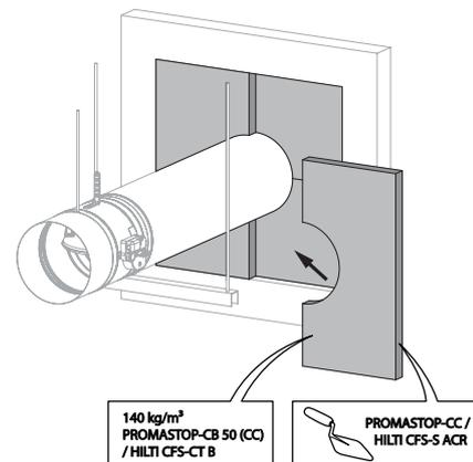
3. An opening with maximal dimensions "A" is made in the wall. For a light partition wall, follow the wall assembly under "Installation in flexible or rigid wall - Sealing with fire resistant rigid panels of stone wool".
