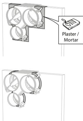
7. Seal the rest of the opening with standard mortar or gypsum.
