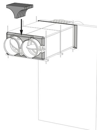
14. Apply rigid stone wool panels ( $150 \text{ kg/m}^3$ ) to a depth of 150 mm to seal the opening at the side with minimal distances.
