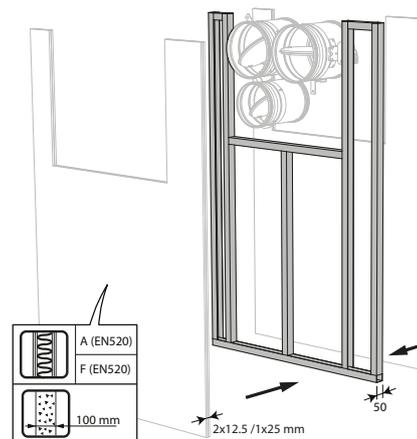
10. Build the drywall and mount horizontal and vertical studs around the opening.
