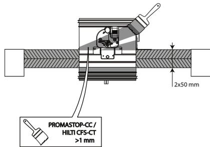
5. For EI 120 S, the casing of the fire damper must be covered with a layer (> 1 mm) of coating (type PROMASTOP-CC / HILTI CFS-CT).
