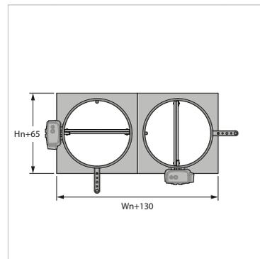
4. The fire dampers may be placed at minimum distance from each other and from the ceiling/floor slab.
