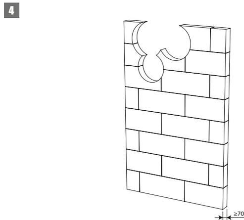
4. Make the necessary openings ( $\leq Dn + 80$  mm) in the wall.
