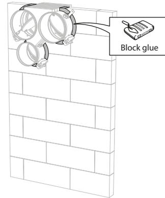
6. Seal the rest of the opening with block glue across the entire wall thickness.
