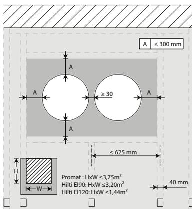
9. For details, please refer to 'Installation in flexible and rigid wall, sealing with rigid rock wool boards with coating'
