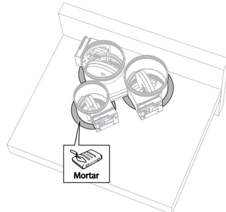
6. Seal the rest of the opening with standard mortar.
