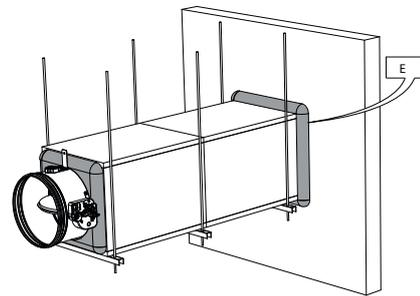
6. The GEOFLAM F / GEOFLAM Light plates stop at a distance of 20 mm from the wall. The free space is filled with fibrous plaster. The same filling is applied to seal off the connection between the GEOFLAM F plates and the damper casing.
