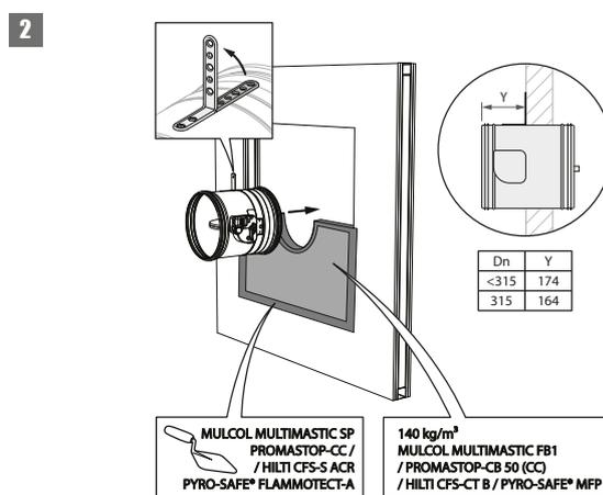
1. For flexible walls, provide horizontal and vertical studs around the opening. Exception: for fire resistance EI60S/EI90S and if sealing with Promastop or Hilti type boards, it is not necessary, from a fire technical point of view, to provide studs around the opening.
