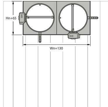
8. The fire dampers may be placed at minimum distance from each other and from the ceiling/floor slab.
