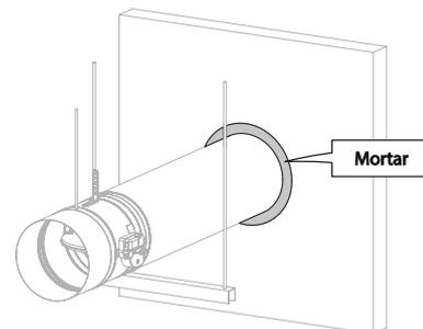
3. An opening with maximal dimensions "A" is made in the wall. The fire damper is mounted remote from the wall at the end of a metal duct. The fire damper is supported by a clamping ring of the same diameter as the damper, held in place by threaded rods "C". The duct is supported every 1500 mm.
