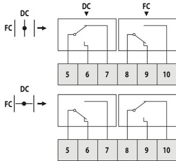
DC: Switch open position fire damper
