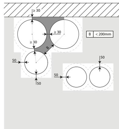
4. The dampers can be installed at a minimum distance (≥ 30 mm) from an adjacent wall or from another damper.
