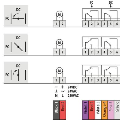
DC: Switch open position fire damper
