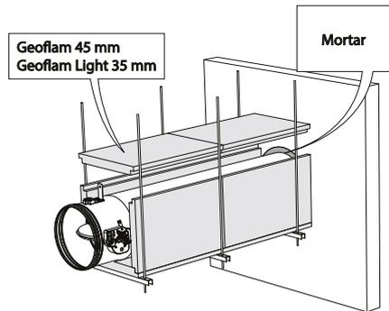
5. The opening around the duct is sealed with standard mortar. The duct is covered with 45 mm thick GEOFLAM F plates or 35 mm thick GEOFLAM Light plates "G". The plates adhere to each other with glue and fibrous plaster "E". The damper casing is also covered on a length of 171 mm.
