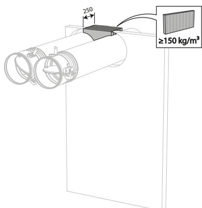
11. Apply rigid stone wool panels ( $150 \text{ kg/m}^3$ ) to a depth of 250 mm (wall thickness + additional at the rear side of the wall) to seal the opening at the side with minimal distances.
