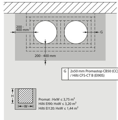
8. The dampers can be installed at a minimum distance from an adjacent wall/floor or from another damper.
