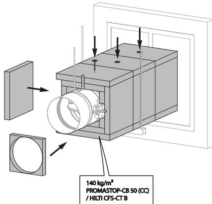
5. The duct is covered over its entire length with stone wool plates "G". To adhere to the duct, the plates are completely coated on one side with fire resistant coating and affixed to the duct with steel screws and washers "E".
