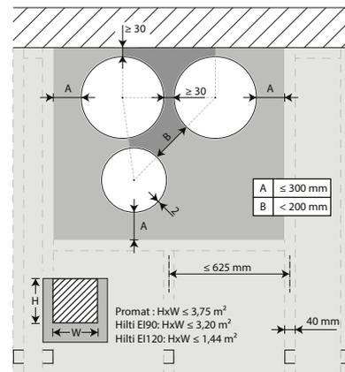
8. The dampers can be installed at a minimum distance ( $\geq 30$  mm) from an adjacent wall or from another damper.
