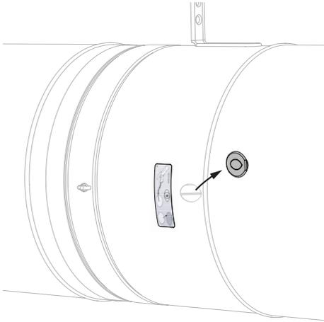
1. An inspection opening (only available when ordering the 'UL' option) allows the position and condition of the damper to be visually determined with an endoscope. For fire dampers equipped with the ONE mechanism, it is also possible to carry out this camera inspection through the opening of the fusible link.
