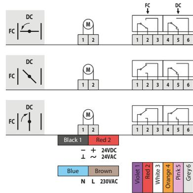
DC: Switch open position fire damper
