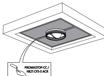
3. The joints on these 2 layers must be installed staggered and covered all around the edge with coating (type PROMASTOP-CC / HILTI CFS-S-ACR).
