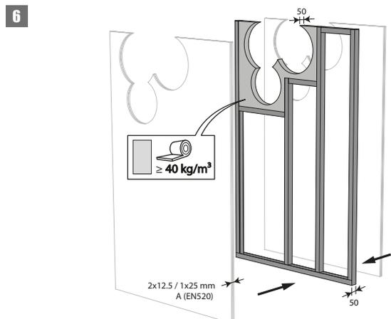
6. Build the drywall and foresee horizontal and vertical studs around the opening.
