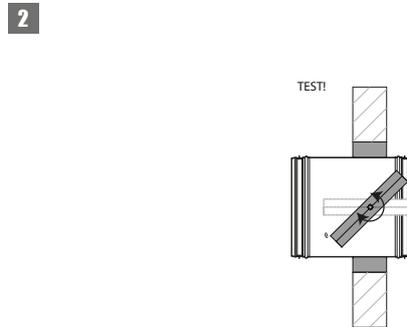
1. Seal the fire damper with a gypsum-based block glue.
