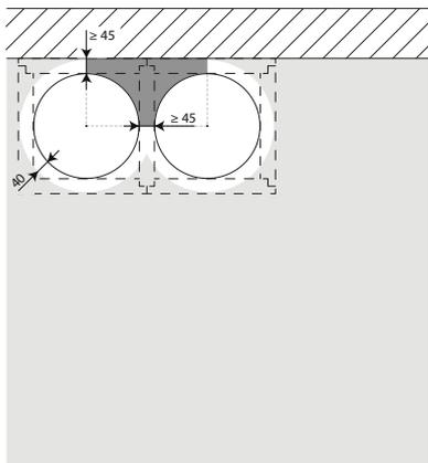
9. The dampers can be installed at a minimum distance from an adjacent wall or from another damper.
