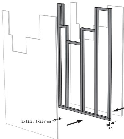
5. Build the drywall and mount horizontal and vertical studs around the opening.
