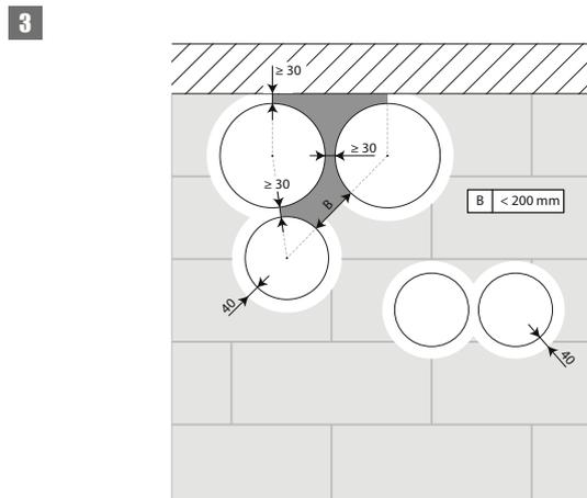
3. The dampers can be installed at a minimum distance from an adjacent wall or from another damper.
