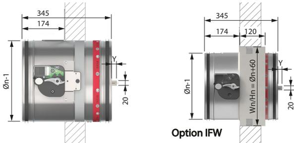
Exceeding damper blade: 20 mm for ØDn 315 mm
