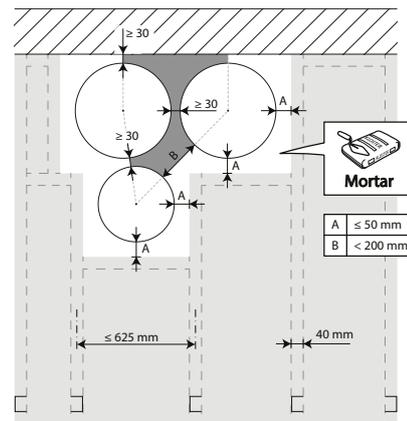
4. The dampers can be installed at a minimum distance ( $\geq 30$  mm) from an adjacent wall or from another damper.
