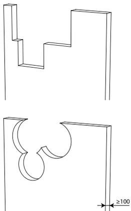
5. Make the necessary openings ( $\leq D_n + 100$  mm) / ( $\leq D_n + 80$  mm) in the wall.
