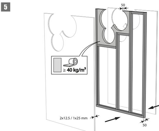
5. Build the drywall and mount horizontal and vertical studs around the opening.
