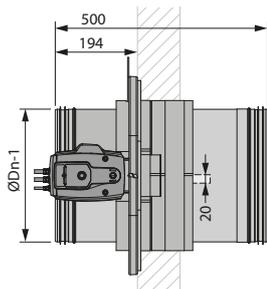
Exceeding damper blade: 20 mm for ØDn 315 mm
