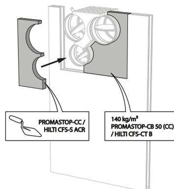
12. Seal the rest of the opening with 2 layers of 50 mm-thick coated rigid mineral wool panels (see above).
