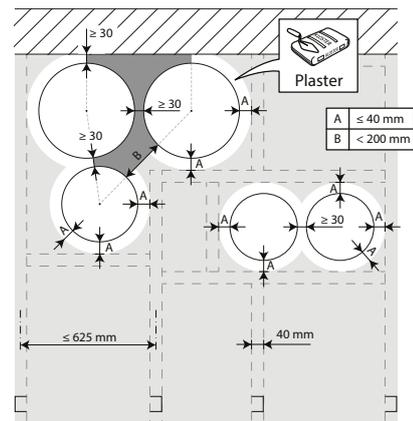
4. The dampers can be installed at a minimum distance ( $\ge 30 \text{ mm}$ ) from an adjacent wall or from another damper.
