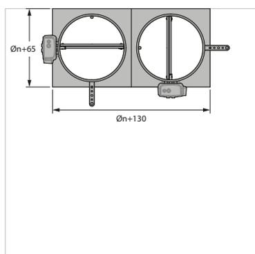
9. The fire dampers may be placed at minimum distance from each other and from the ceiling/floor slab.
