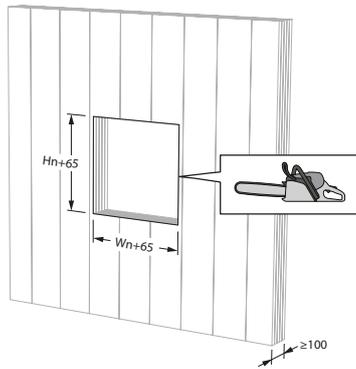
1. Saw out the installation opening on site if not provided.
