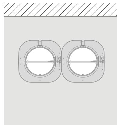
6. The dampers can be installed at a minimum distance from an adjacent wall or from another damper.
