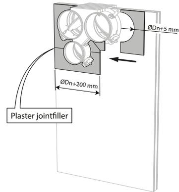
8. Apply cover plates (gypsum plasterboards) to finish the surface at both sides.
