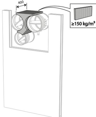
11. Apply rigid stone wool panels ( $\geq 150 \text{ kg/m}^3$ ) to a depth of 400 mm (150 mm on the mechanism side of the wall) to seal the opening at the side with minimal distances. The surface of this sealing is set between the axes (centres) of the dampers.
