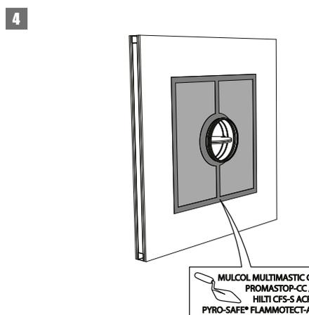
3. The joints on these 2 layers must be installed staggered and covered all around the edge with coating (type PROMASTOP-CC / HILTI CFS-S-ACR / Mulcol Multimastic SP / PYRO-SAFE® FLAMMOTECT-A).
