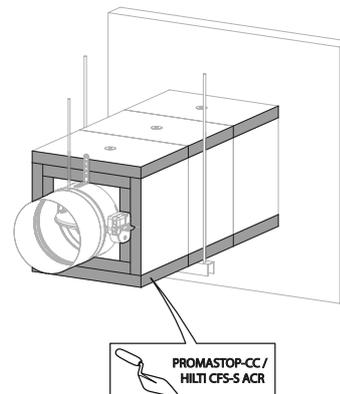
6. The joints between the plates, between the wall and the plates as well as the screws and washers are filled with coating PROMASTOP-CC / HILTI CFS-S ACR.
