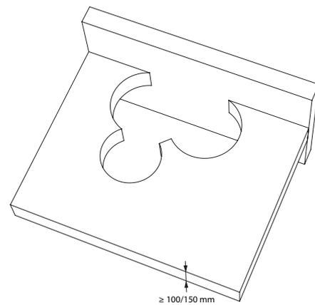
3. The dampers can be installed at a minimum distance ( $\geq 30$  mm) from an adjacent wall or from another damper.
