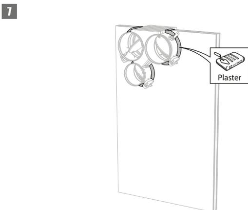
7. Seal the rest of the opening with standard gypsum across the entire wall thickness.
