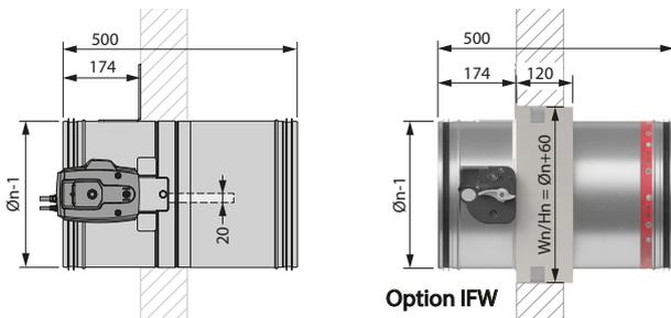
Exceeding damper blade: 20 mm for ØDn 315 mm
