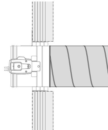
4. With a wall thickness  $\geq 135\text{mm}$  ( $\geq 290\text{mm}$  for CR120-L500), the connecting duct falls within the wall.
