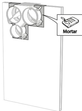
7. Seal the rest of the opening with standard mortar across the entire wall thickness.
