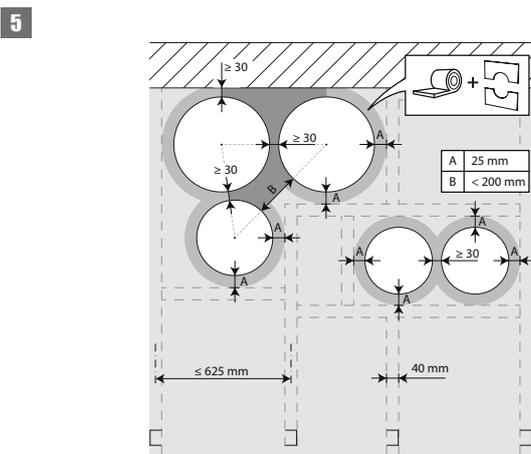
5. The dampers can be installed at a minimum distance (≥ 30 mm) from an adjacent wall or from another damper.
